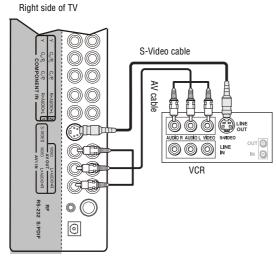
3 Connect the audio plugs on the AV cable to the AV1 IN AUDIO-L and AUDIO-R jacks on the right side of your TV.
